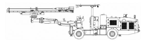
CYTJ45A Hydraulic drilling jumbo is used for underground tunneling construction in metal mine and other small and medium sized cross section tunneling work. Due to advanced all hydraulic drilling system, and anti-jamming function, the jumbo features of rapid drilling speed, and high efficiency. Compact structure and flexible tramming could greatly improve working environment and gets efficiency and qualified development.
