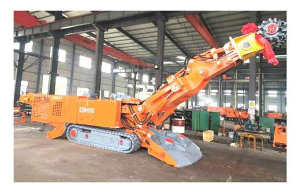
EBH160 cantilever road header is designed by KAMACH MINING with multifunction hydraulic-control cantilever road header.
