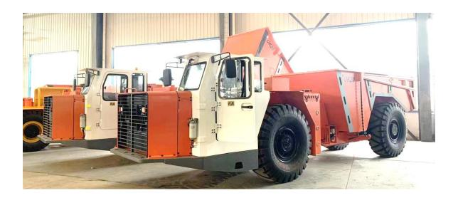
UK-15 Underground MineTruck is used together with WJ-3 or WJ-4 UG production loader. Power supply is emission tier 3 water-cooled diesel engine, to reduce the fuel consumption, and exhaust.
